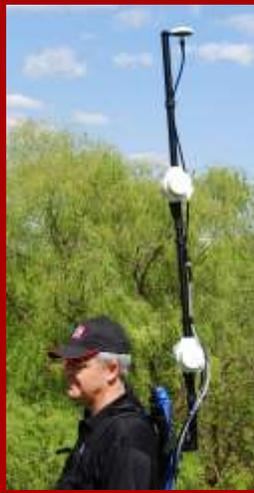
**GEM's GSM-19 system with integrated GPS option. This system provides a light weight, low cost solution for walking use. It includes a "Walking" mode that enables continuous readings as well as navigation resulting in high productivity surveys.**
