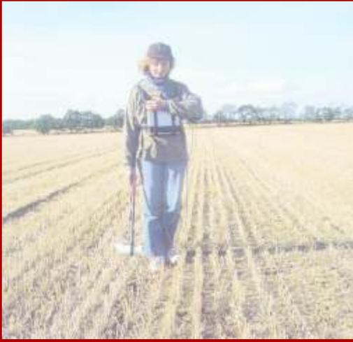
**GEM's GSM-19 system in use in Denmark. This system provides a light weight, low cost solution for walking use. It also includes a "Walking" mode that enables nearly continuous coverage with resulting high productivity surveys. GEM Non-magnetic cart shown below for near surface surveys.**
